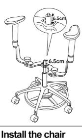
Step 7: Take away temporarily the seating cushion (7), and put the installed arm-rest (5+6) on gas cylinde(4), istalled with (1+2+3), make sure to reserve 6.5-8.0cm on top of the cylinder and fasten it with 2 screws
