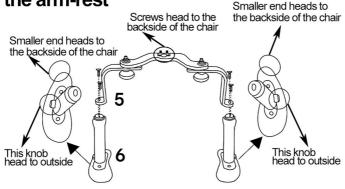
Step 6: Put the arm-rest PU part (6) upside down on a desk, remember to put the small end of the part to the backside of the chair, and the two knobs head to the outside . Put on the arm-rest metal part (5) and fasten with 4 screws.
